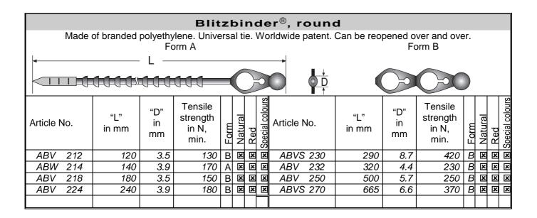
The Allplastik-Blitzbinder® quick fasteners made of premium quality polyethylene have a special closure which, when combined with a round profile, guarantees maximum strength and reliable closing and can also be opened again at any time. In addition to its function as a fastener, the dual closure design of the Allplastik-Blitzbinder® quick fasteners allow a hanging loop to be formed.
